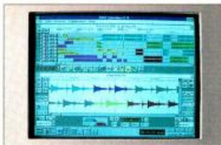
SADiE from Studio Audio and Video is a Windows-based system featuring fast, user-friendly editing and mixing of up to eight tracks.
