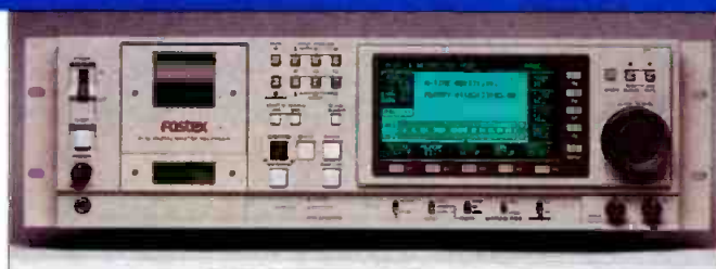
The Fostex D-30 features a super twist display like those found on some laptop computers. It includes many advanced features, such as time code, off-tape monitoring, scrubbing, edit previewing, auto-cuing to first audio, instant start and RS-422 control.
